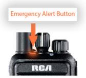
trigger an alarm by pressing this orange button. Immediately, the RCA two-way radio sends out a voice and/or radio identity to notify specific individuals of an impending emergency. This drastically reduces response times and significantly contributes to a safer environment.
