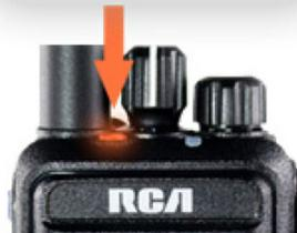
trigger an alarm by pressing this orange button. Immediately, the RCA two-way radio sends out a voice and/or radio identity to notify specific individuals of an impending emergency. This drastically reduces response times and
